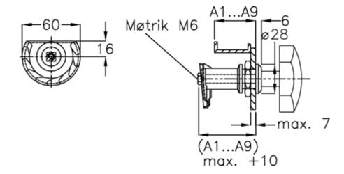
Door + frame thickness = 52-60 Measure type = A8
